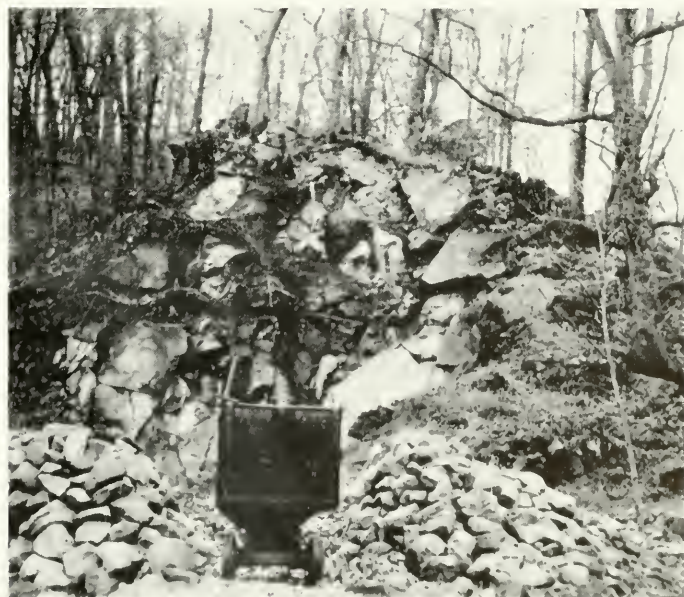
FIGURE B.—Small olivine quarry in large residual boulder of dunite.
